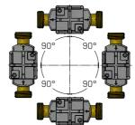
The flow sensor can be mounted horizontally, vertically or at an angle.
