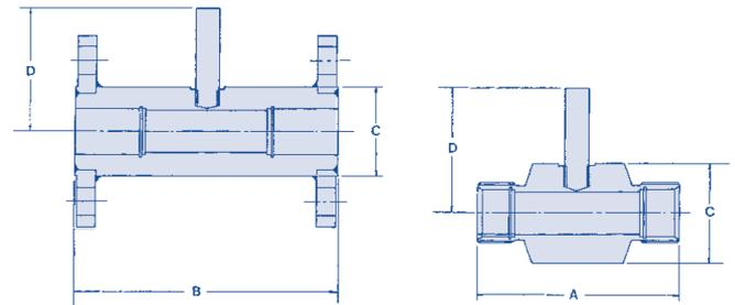
**Allow an extra 50 mm height on dimension 'D' for pick off coil connector.**
