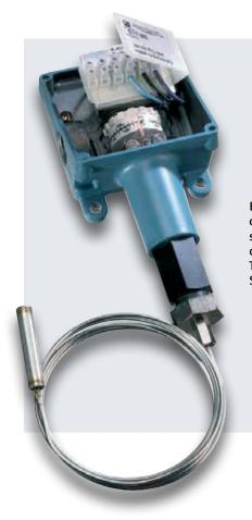
E117 bulb and capillary temperature switch shown with cover removed. Terminal block with SPDT switch output.
